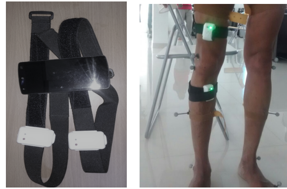
(a) Portable System: EXL-S3 IMU Sensors with smart phone. (b) Placement of IMU sensors.
