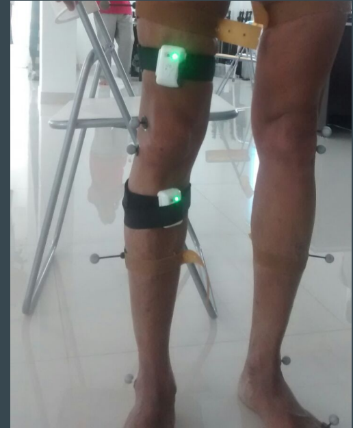
Placement of Sensors on Thigh and Shank of right Leg. (along with Optical Markres).
